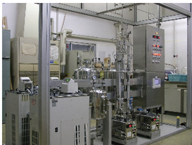
Figure 4. Picture of the pilot plant for the halogen–magnesium exchange reaction of BPFB and EtMgBr.
